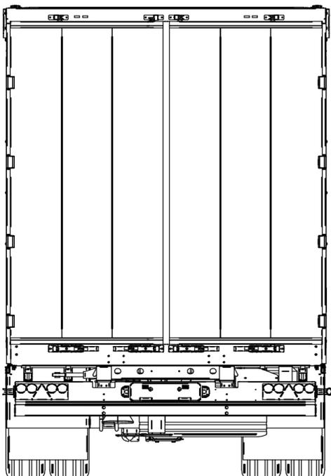
Rear frame is composed of 2 pillars with 40 mm width and made of high strength steel. Magna2 doors have only 3 vertical profiles of 420 mm; their design and strength have no comparison in the market. You can select different lock types.
