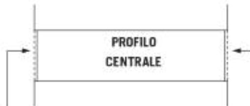
*The central profile is slightly shorter (2 mm) than the outer profiles to avoid interference during fitting the top and bottom rails. It is, therefore necessary to ensure that it does not extend on either extremity.*
